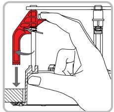
4.4 With the frame connected it may be lifted up into the ceiling aperture. On speakers with tilting tweeters, correct frame orientation must be established at this stage: the red arrow on the frame flange should be pointing towards the listening area.
