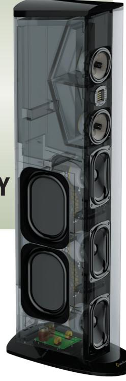
Handling the high frequencies is a folded ribbon tweeter. GoldenEar says that rather than pumping air in the manner of a regular cone-based tweeter, this 'squeezes' the air to pressurise it, using a high temperature film in a strong magnetic field generated by neodymium magnets.
