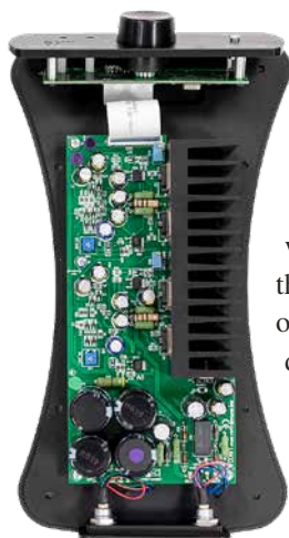
The speed control unit, in which the sine waves for the AC motor are generated by means of a DSP, was a completely new development.
