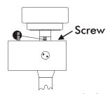
With the aid of a good magnifying glass adjust the needle until it is vertical in the groove (i.e. perpendicular to the record's surface). Ideally this should correspond to the top surface of the cartridge body being parallel to the record surface.
