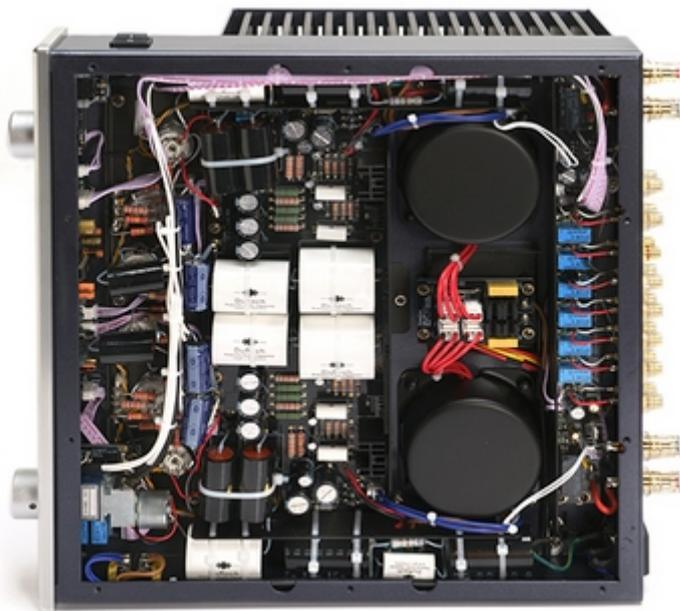
Removing the bottom cover is a visual feast for the parts geek/aficionado. A cursory look reveals an expensive ALPS volume pot, along with resistors and capacitors from Nichicon, Rubycon, Kemet, Takman, DuRoch, and others. This is the kind of stuff that one usually finds lurking in amplifiers costing 3-5 times as much.
