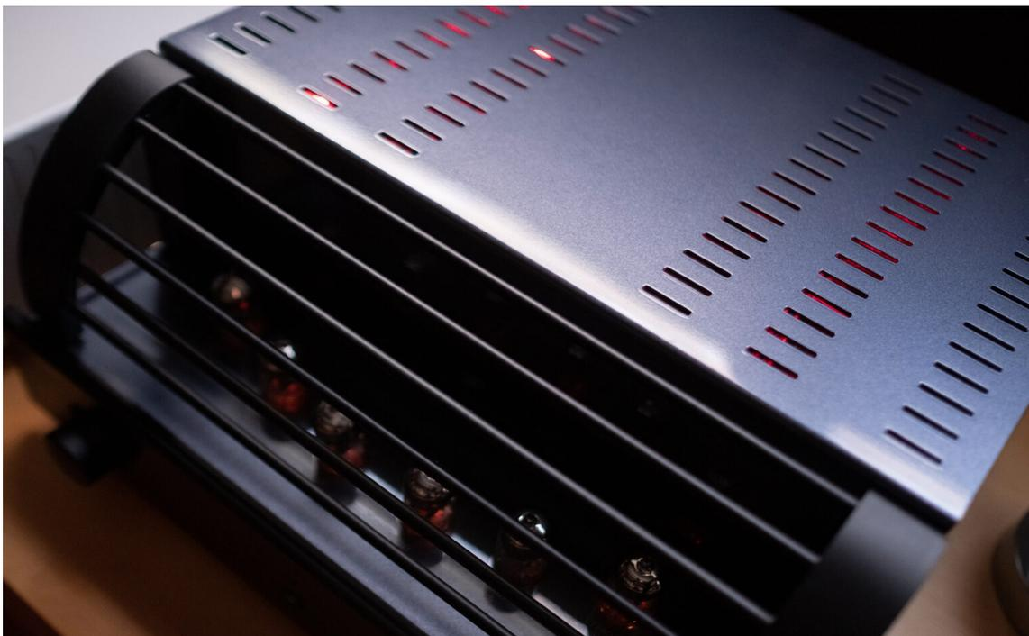
The EVO 300 Hybrid Tube Integrated Amplifier is built like a tank (for music) and is about as heavy, weighing a lift-with-your-legs 68.3 lbs. which feels much heavier today than it did in 1998. An curved removable tube cage is provided to keep those 12AU7s and you safe, while the front face comes in silver and black and sports two control knobs for input selection and volume and a 1/4" headphone jack.
