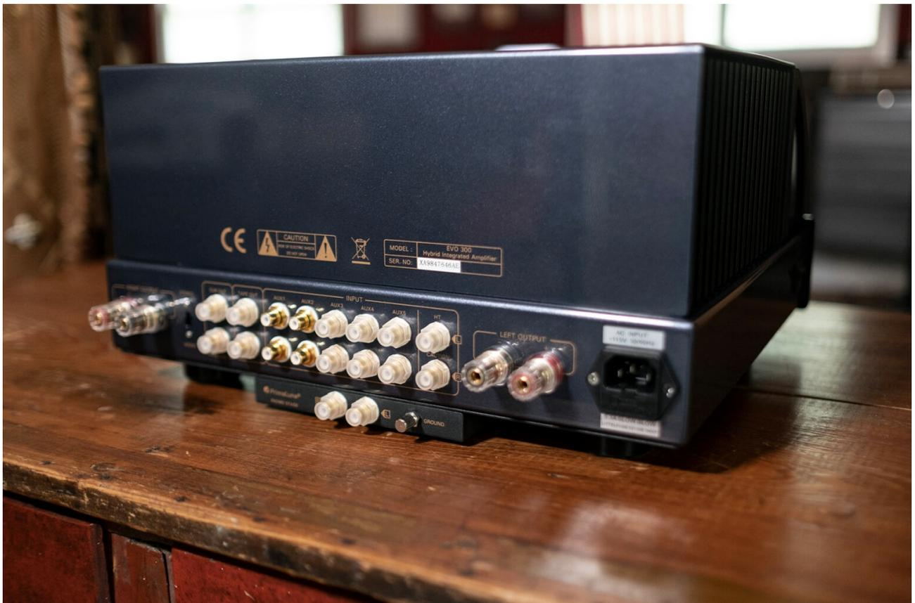
The EVO 300 offers 5 stereo RCA inputs, a stereo RCA Home Theater Bypass input, a single set of speaker binding posts, RCA Stereo/Mono Subwoofer out, Stereo RCA Tape Out, and a 1/4" Headphone jack mounted up front that is powered by the same internal amp as the speakers (look ma, no op-amps). There's also an optional belly-mounted MM phono stage, absent on the review sample (the case is there, the optional phono board isn't in it).
