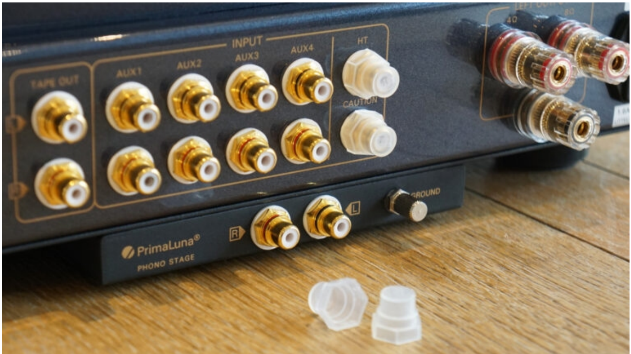
Optional moving-magnet phono stage sits in a separate shielded case that's bolted to the amp's underside. Dust caps are a great inclusion to keep the input sockets clean and protected when not in use
