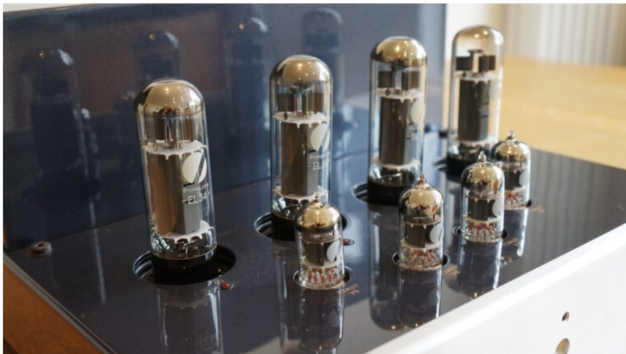
Four 12A7 valves (front) are dwarfed by a quartet of EL34s, which can be swapped with alternatives such as KT88 types, should you want a different sonic flavour.
