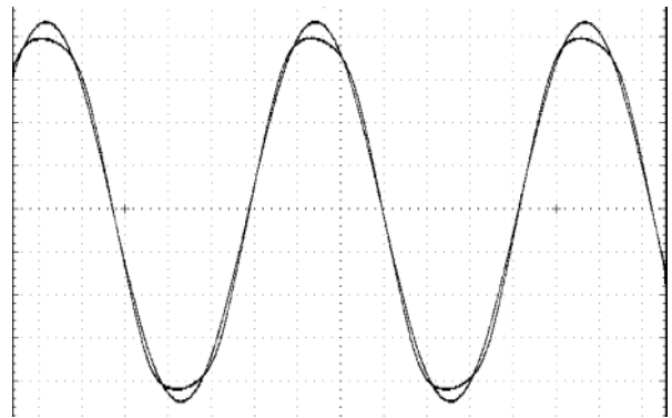
This trace shows the signal level at the clip threshold with the peaks being slightly rounded or “soft clipped” which will add warmth and strong 2nd harmonics.
