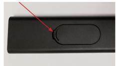
Install the CR2032 with the positive (+) side facing up in the slot sliding the battery under the small lip by the "+" symbol.
