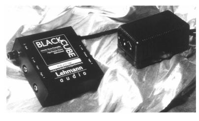
Enter Black Cube, new, improved and kicking booty in a town near you! This newer version uses a circuit board with checkered grounding plane versus solid. On the phono board itself the older Analog Devices chip has been replaced with a better Burr Brown unit. There were also some minor parts change in the power supply while the latest big change is the usage of a non-magnetic aluminum chassis instead of steel. The use of
