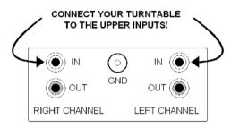
Now connect a good pair of unbalanced interconnects from the outputs to a pair of line level inputs on your amplifier.
