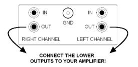
Make sure the connectors are pushed all the way in, but **beware of using excessive force** as you might cause cracks in the circuit board. If connectors are too tight or too loose, the music will suffer. If you need advice on how to adjust your connectors for optimal pressure, please contact us, your dealer or our forum on the internet!
