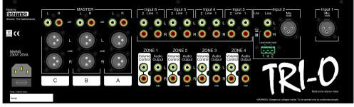
Channel 1 has a talk-over circuit to improve the speech intelligibility. This circuit, which is triggered by the microphone signal from channel 1 (i.e. it is voice-activated), ensures that this signal overrides all others. The talk-over function can be disabled with the TalkOver switch on the front.
