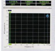
The Evolution produced minuscule amounts of distortion, measuring just 0.002% in the midband at 1 Watt, and the same close (-1dBV) to full output. At high frequencies distortion rose little, measuring 0.01% second harmonic only, our analysis shows, and this distortion pattern remained absolutely stable as output increased, suggesting the amplifier will sound smooth in its treble and free of harshness. The low level of distortion and its consistent pattern suggest the output stage works better
