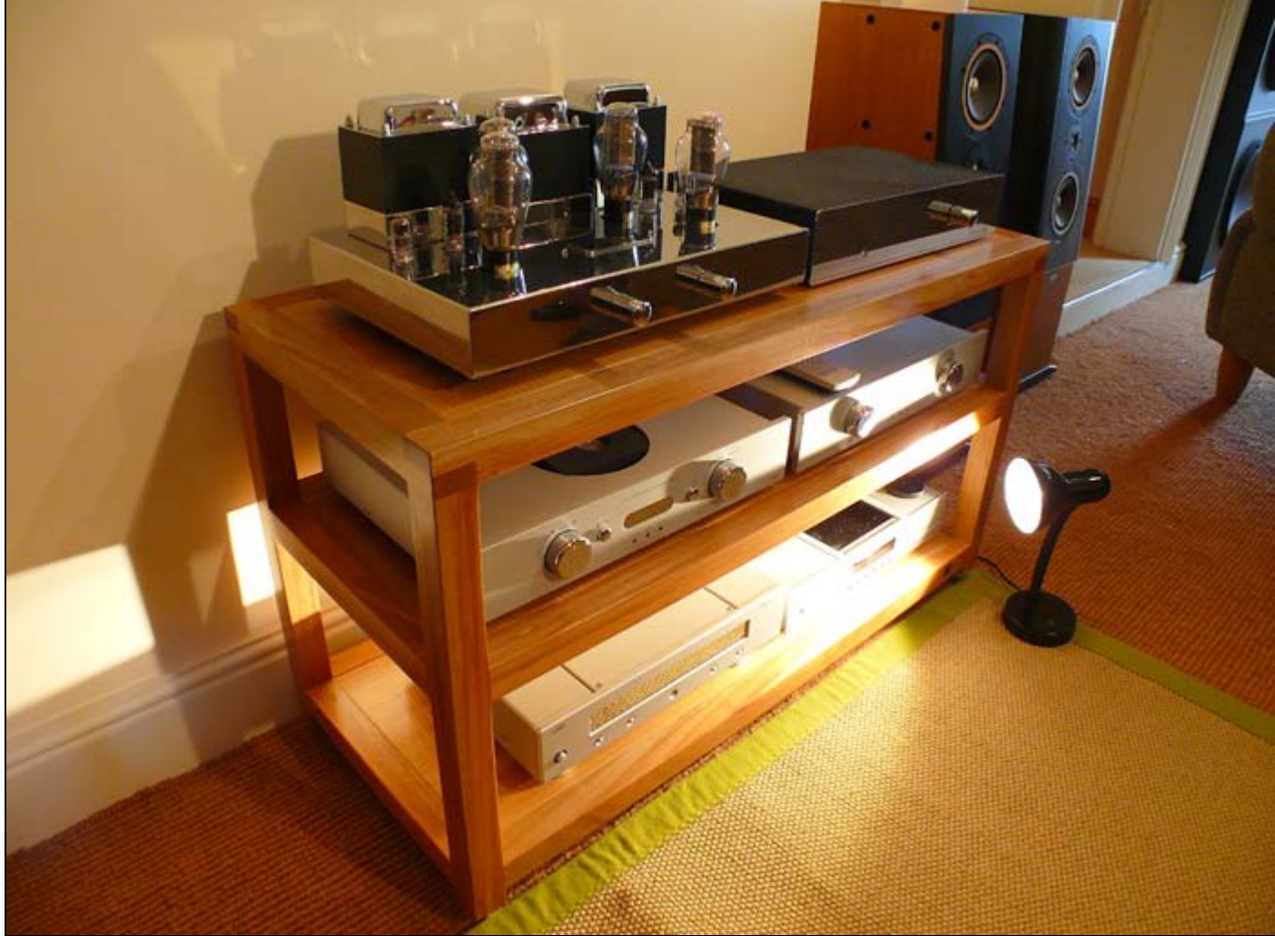
An Art Audio Argento amplifier from Tom Willis who lives 10 minutes away. Definitive Audio rewires this 300B parallel single-ended amp with Kondo, replaces the signal coupling caps, the stock pot and adds a proprietary outboard filament supply transformer with Kondo umbilical.
