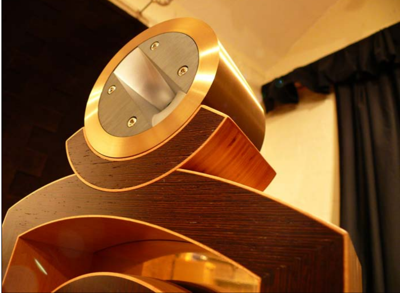
The 45° outwards rotation of the super tweeter is locked and optimized for widest dispersion. Unlike the production pair, the wood finish on this first pair was open grain.
