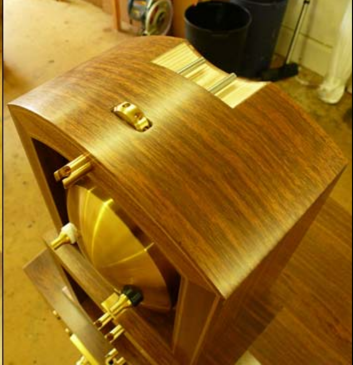
Here is the exposed worm drive assembly for the ultra tweeter module.
