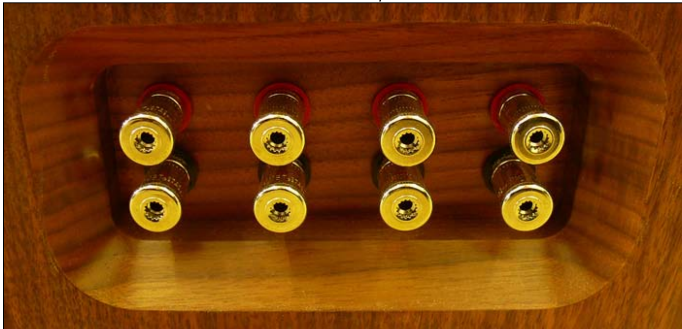
The binding post bay.
