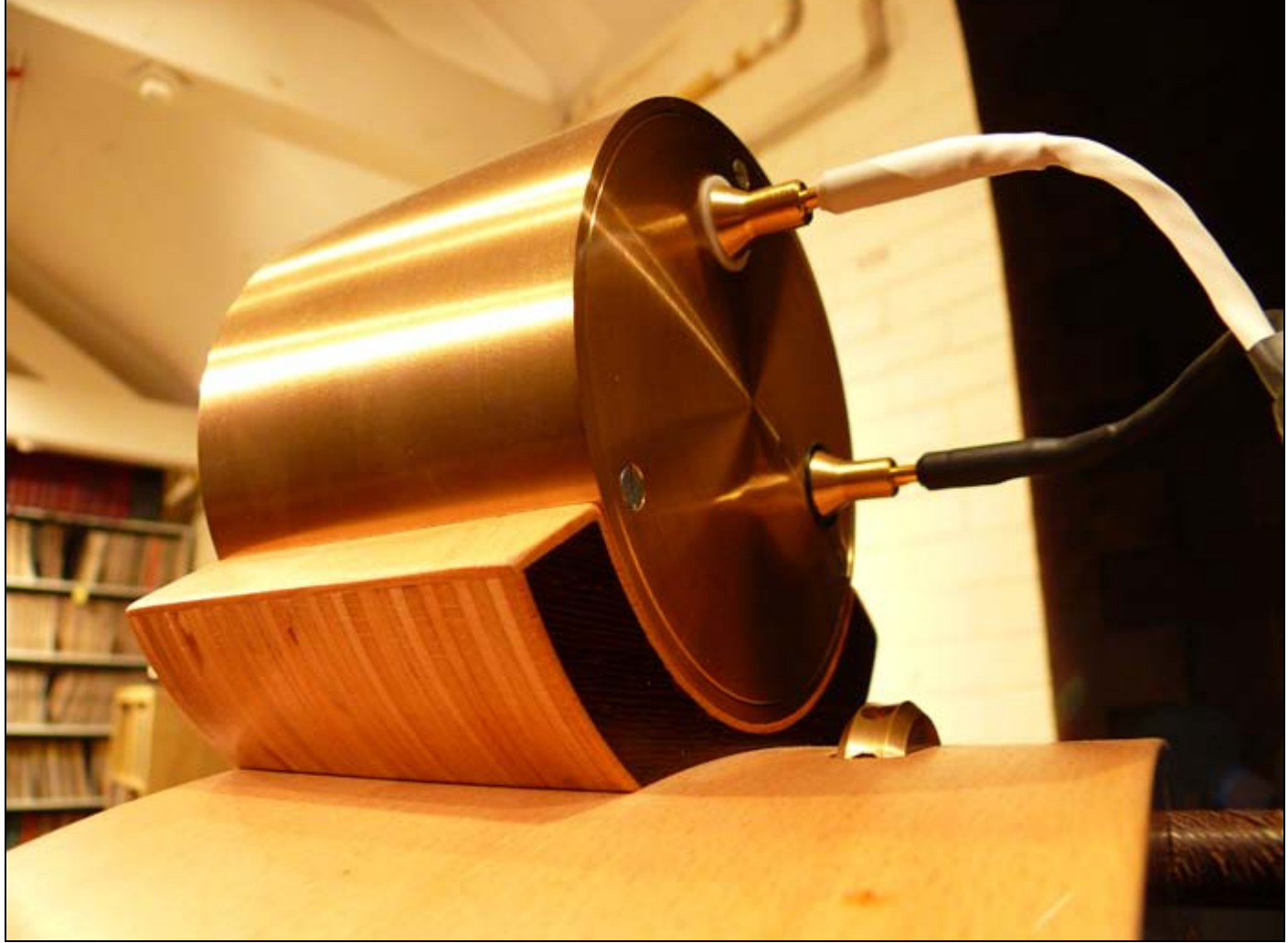
The nested super tweeter with exposed worm drive wheel.
